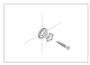
Fix SpinFix button and washer to substrate.
