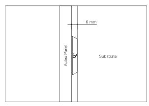
SpinFix clips create a 6 mm air gap for added acoustic performance.
