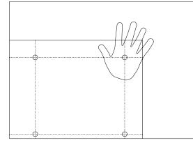
Press panel onto SpinFix clips to mark the fixing points.
