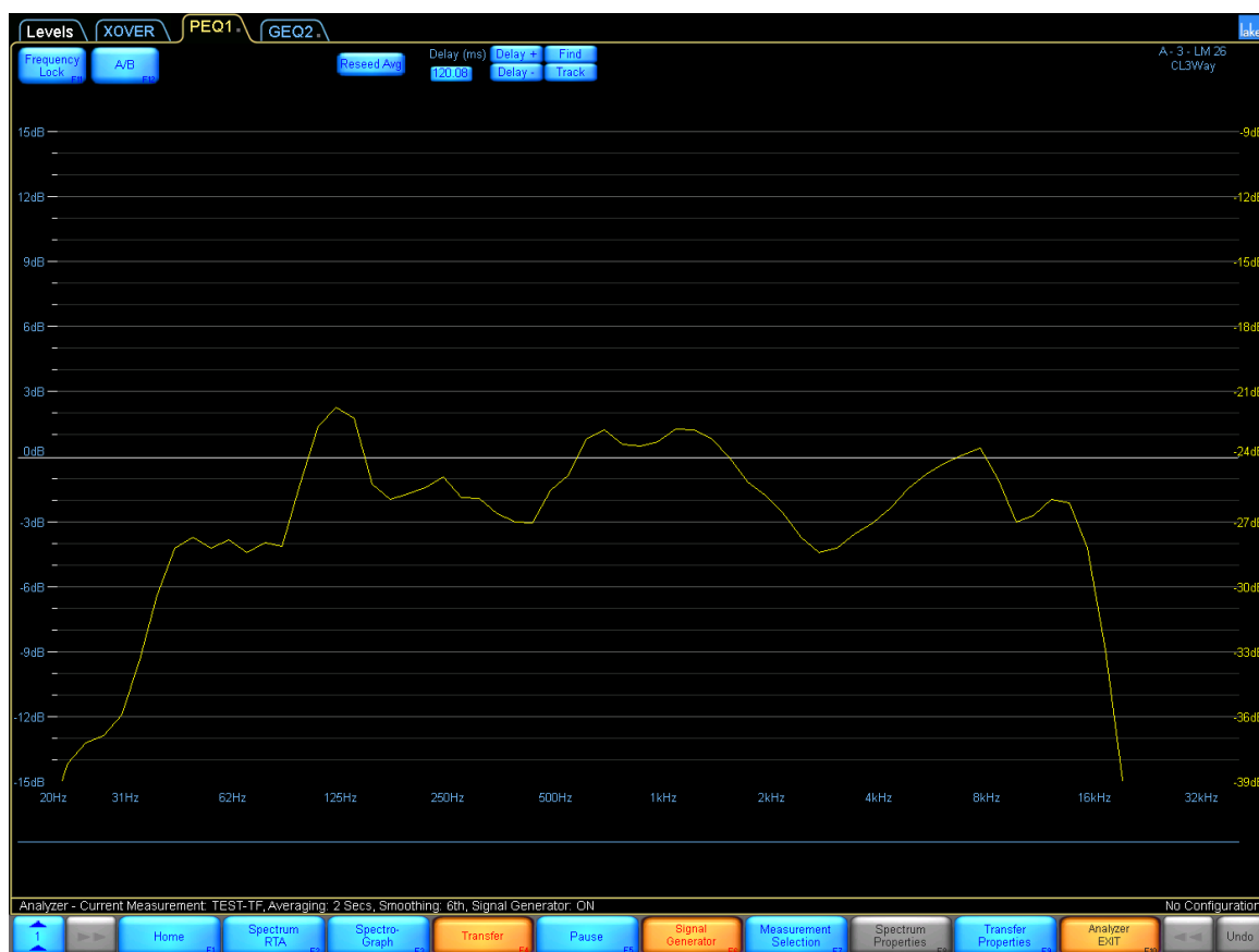
Figure 18-12: Transfer function measurement mode
