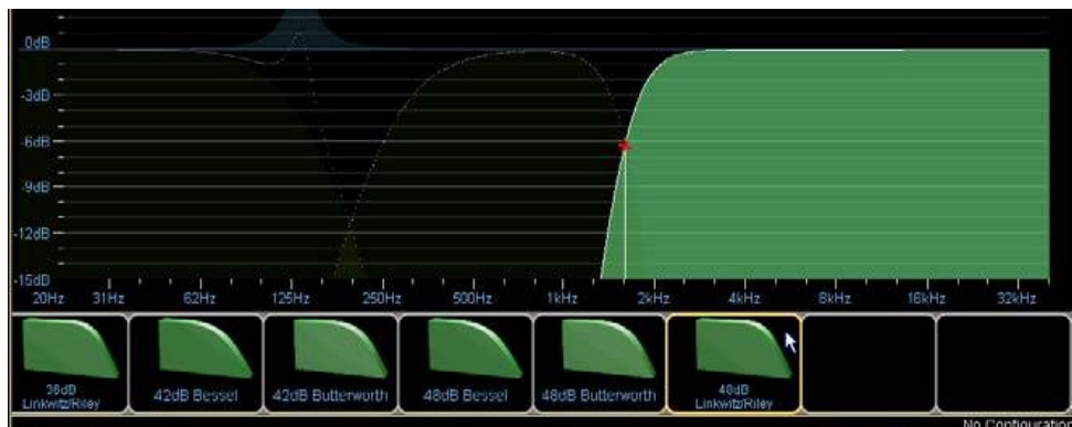
Figure 4-49: Changing the crossover slope
