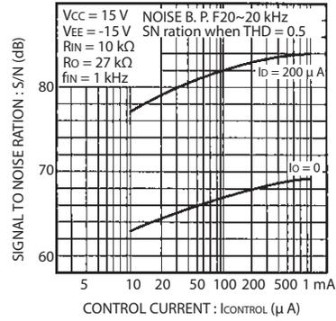
Fig.4 SN ratio - control current characteristic
