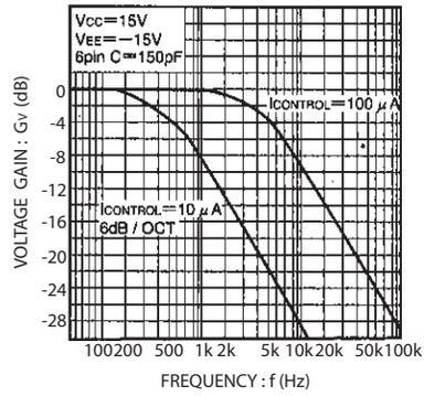
Fig.7 Low pass filter characteristic
