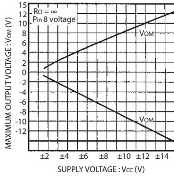
Fig.5 Maximum output voltage - power supply voltage characteristic
