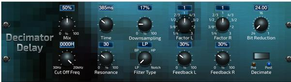
This is a delay effect including a decimator unit in its chain. It will decimate the sound by reducing the sampling frequency and the bit-depth. The Decimator Delay is a creative tool that can be used in many ways, from emulating the aliasing noise, found in older samplers, to generating complex, low-fi and rough delay lines.
