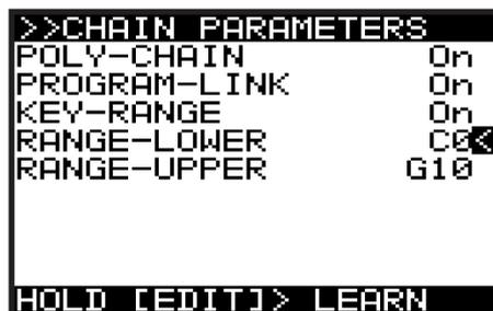
3. To navigate the options in the CHAIN PARAMETERS menu, use the BANK/UP or BANK/DOWN switches.
