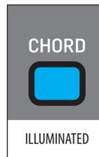
When the CHORD switch is pressed, it will illuminate, and the chord screen will appear in the display. (If no chord is currently stored, then the switch will flash.)
