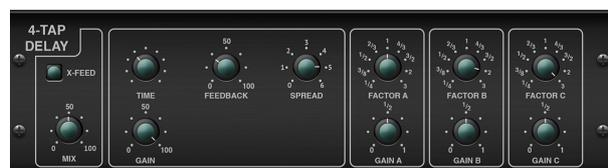
The 4-Tap Delay provides 4 stages of delay with independently adjustable gain and rate, allowing unique syncopation to be created in the layered repeats.
