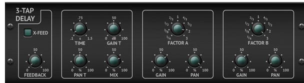
Sometimes called a 3-Tap Delay, the Triple Delay provides three delay stages with independent frequency, gain, and pan controls. Create time-based echo effects with the Triple Delay to increase the sense of stereo separation.
