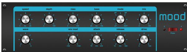
The Mood Filter uses an LFO generator and an auto-envelope generator to control a VCF (voltage-controlled filter), as well as a side chain function where the channel B signal controls the envelope of channel A.
