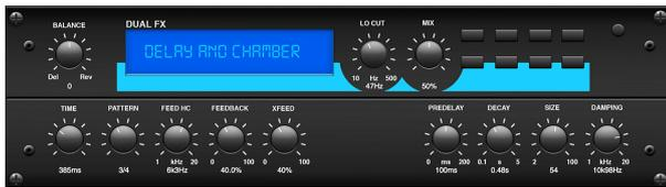
Here we have combined Delay and Chamber reverb, so a single device can provide a variety of delay settings, plus add just the right type and amount of reverb to the selected signal. This device only uses one FX slot. (Inspired by the Lexicon PCM 70.)
