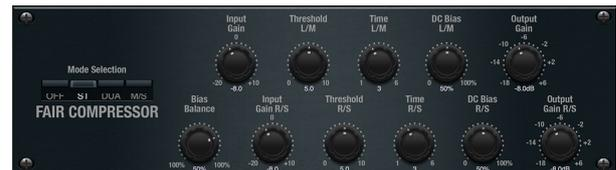
This model of a Fairchild 670 delivers some of the finest colorations in compressor history. The two paths L/M and R/S both have the same functionality. The controls include input GAIN, THRESHOLD, TIME and DC BIAS (which controls the ratio and knee of the compression curve). There is also a BIAS BALANCE which can help accentuate attacks. There are modes available for dual, stereo-linked, or mid/side operation via the MOD control.
