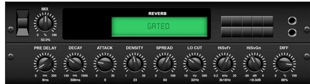
This effect was originally achieved by combining a reverb with a noise gate. Our gated reverb creates the same impression by a special shaping of the reverb tail.
