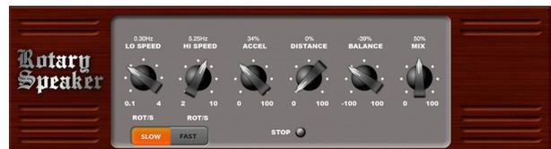
Rotary Speaker emulates the sound of a Leslie rotating speaker. The Rotary Speaker provides more flexibility than its electromechanical counterpart, and can be used with a variety of instruments, and even vocals, to create a whirling, psychedelic effect.
