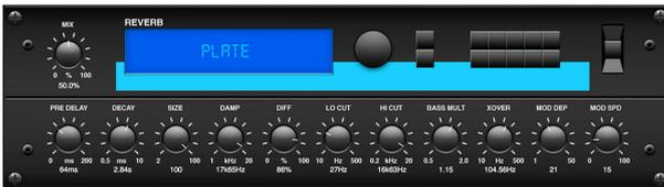
A plate reverb was originally created by sending a signal through a transducer to create vibrations on a plate of sheet metal which were then picked up as an audio signal. Our algorithm simulates that sound with high initial diffusion and a bright colored sound. The Plate Reverb will give your tracks the sound heard on countless hit records since the late 1950s. (Inspired by the Lexicon PCM-70.)
