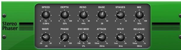
A Stereo Phaser, or phase shifter, applies multiple STAGES of modulated filters to the input signal to create a “notch” in the frequency response, and then applies a MIX with the original for a “swirling” effect. Use the Stereo Phaser to add a “spaced-out” sound to vocal or instrument tracks.
