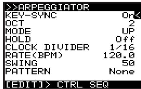
**Note:** In the ARP/SEQ EDIT menu there are three pages: ARPEGGIATOR, CONTROL SEQUENCER, and ARP SETTINGS. This section covers the ARPEGGIATOR menu. To cycle through the pages, use consecutive presses of the EDIT switch. The bottom line of the screen will show guidance to the next page.
