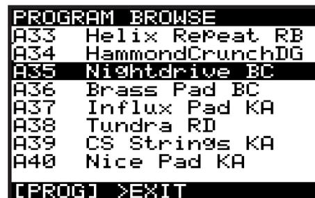
3. When in program browser mode, you can use the rotary knob to scroll through the list of programs. When you stop on a program it will be automatically loaded.
