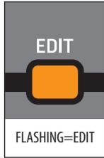
**Shortcut Note:** To quickly change the LFO waveform shape, press and **hold** the LFO EDIT switch, and move the LFO RATE fader.
