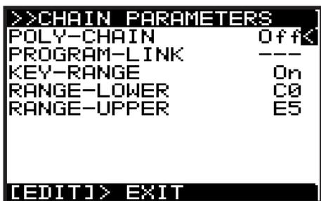
2. Select POLY-CHAIN OFF for each unit. (PROGRAM-LINK is not an available option when POLY-CHAIN is OFF.)
