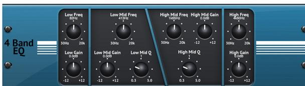
The Midas EQ is a four-band sweep parametric equalizer taken from the Midas Pro X console that allows tonal control of the input signal via the parametric EQ section. The mid bands also have a Q Factor adjustment to tailor the shape of the EQ curve. The four bands are low, low mid, high mid and high. Any combination of the four bands can be used to control the signal.
