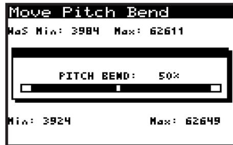
7. To confirm the CALIBRATION of the PITCH WHEEL press the +/YES switch and you will be moved on to the PITCH CENTRE page:
