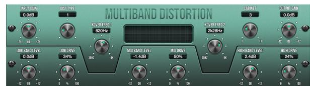
The Multiband Distortion unit, useful for making sound gritty, adding more warmth through saturation, or even enhancing a specific frequency region. There are three bands, adjustable by a 24 dB per octave crossover filter.
