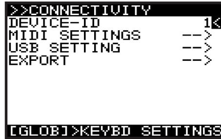
In this menu are all the settings relating to connectivity and communication with external devices, including backing up and restoring programs and data.
