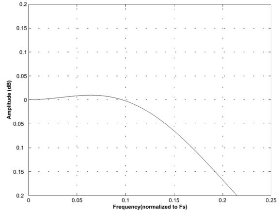
Figure 42. Quad-Speed (fast) Passband Ripple
