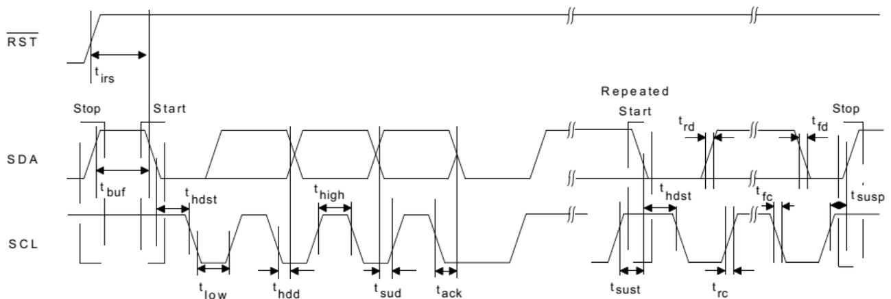
Figure 10. Control Port Timing - I<sup>2</sup>C Format
