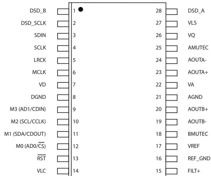
Figure 2. M9000 Pinout Drawing-TSSOP
