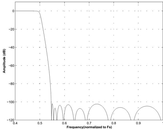
Figure 23. Single-Speed (fast) Stopband Rejection
