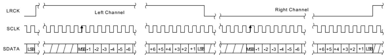
Figure 7. Format 2, Right-Justified 16-Bit Data.
