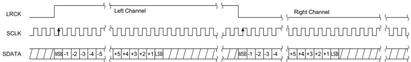
Figure 5. Format 0 - Left-Justified up to 24-bit Data
