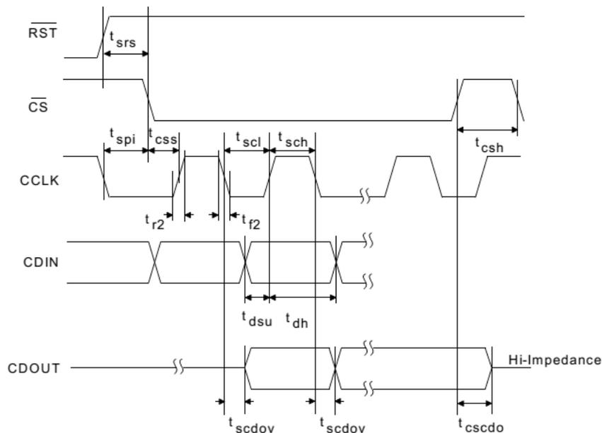
Figure 11. Control Port Timing - SPI™ Format(Read/Write)
