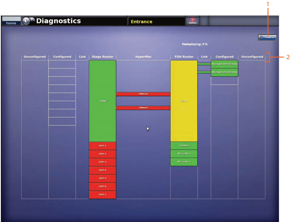
An example of the Diagnostics screen, showing the three types of device condition.
