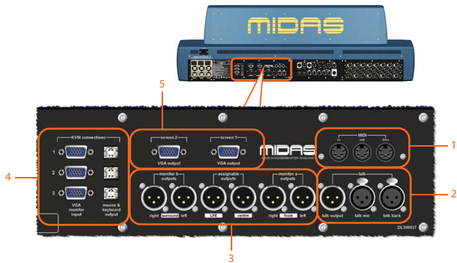
External connections and communications on the rear panel of a PRO X Control Centre
