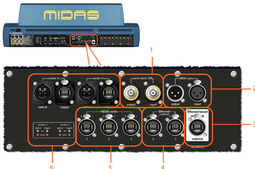
Typical audio, networking and synchronisation connections on the rear panel of a PRO Series Control Centre
