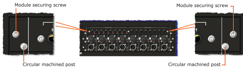
Position of the module securing screw and circular machined post at either end of a module (rear of PRO Series Control Centre)
