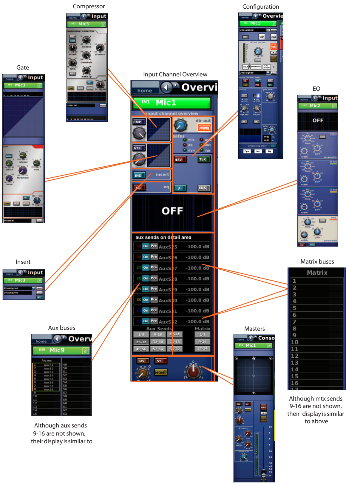
Figure 34: Processing areas available from the input channel overview display
