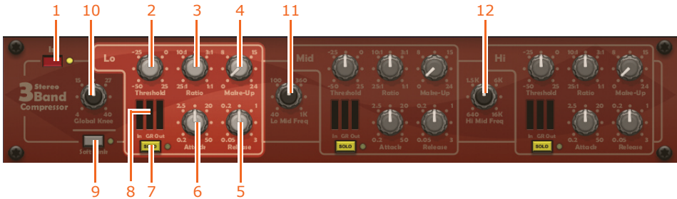
Front panel of the 3-band compressor effect
