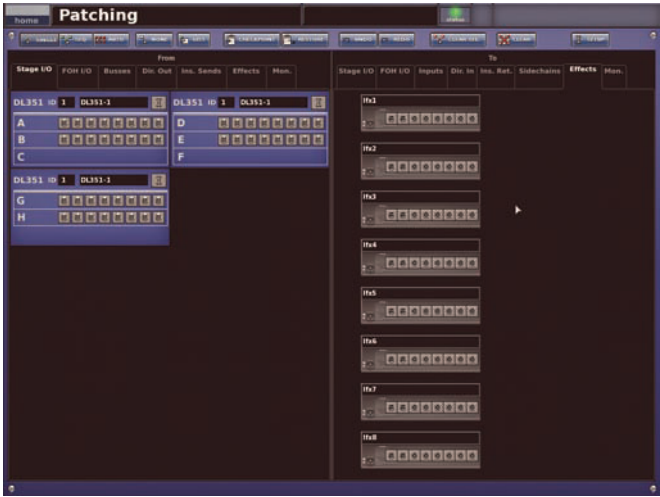
Patching screen showing the location of the effects in the Effects tab of the To section.
