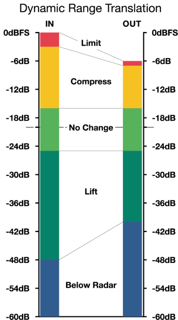
Fig 12. Example of dynamic range re-mapping: From Home Theatre/DVD to Living Room listening conditions ( Fig 1 ).
