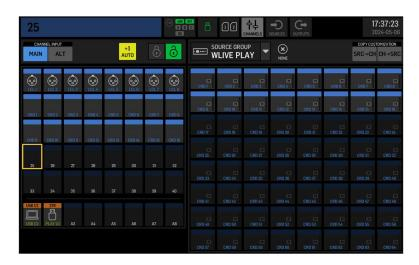
At that point, Channel Strips 9 to 24 can be used to mix the audio data issuing from the first 16 tracks of SD card 1<sup>105</sup>. Channel Strip 1 to 8 can be used to mix the audio data coming from local inputs 1 to 8 at the back of the console, and Aux strips 1 and 2 can be used to mix the audio signals from USB 1 & 2 and the 2 tracks from the USB stick player.
