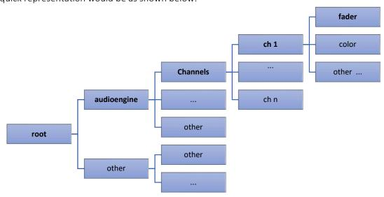
Computers use specific data structures to represent trees. WING uses one of them, based on JSON<sup>6</sup> notation. It is important to know/understand the list of sub-trees (nodes), and leaves (parameters) WING contains as this is how you can access to data. More detail on the WING data set is provided in appendix.
