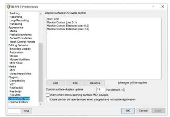
: If the "ignore global bank offsets" flags are **not** checked in the REAPER MIDI surface control setup panels above, using the 4 and 4 WING buttons will enable you to navigate left and right in the REAPER tracks if more than 24 REAPER tracks are available.
