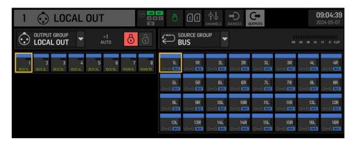
Changing the output routing is made from the ROUTING→OUTPUTS screen, with first clicking on the OUTPUT GROUP of interest to select the first physical destination you want to assign a WING signal to.
