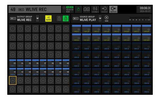
The audio data used for our mix will be recorded to SD card 2, from SD card 1 (only when engaging record on SD card 2 and play on SD card 1, of course).
