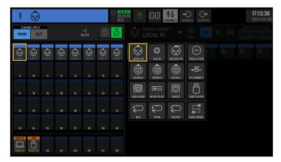
SOURCES include actual HW sources and logical audio paths such as BUS, MAIN, MATRIX and USER SIGNAL, which are either the result of partially mixed audio or a specific/customized selection of Source in the case of USER SIGNAL.
