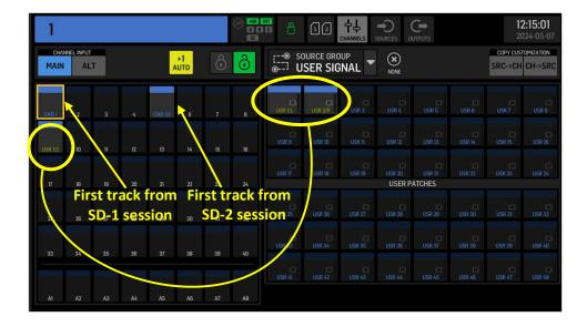
That same USER SIGNAL 1 can also be used as a SOURCE for an OUTPUT, such as for example to record into a DAW on a PC using a USB connection, as a single stereo pair into USB 1&2.
