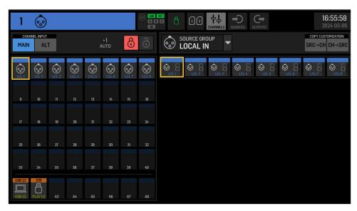
There are two routing options: MAIN and ALT. Both serve the same purpose and can be selected within Channel Strips; There are therefore two routing tables available at the desk.
