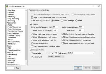
With the settings above, and WING DAW mode setup to USB MIDI, MUC+2xExtenders, you now have a 24 channel strips DAW surface control to manage REAPER tracks (Volume, Solo, Select, Mute) from your WING, and vice-versa (i.e. changes made on a surface (WING or REAPER) will reflect on the other); REAPER tracks' Pan control can be achieved using the 4 rotary knobs in the WING control zone, situated just below the "Custom Controls" silkscreened text.
