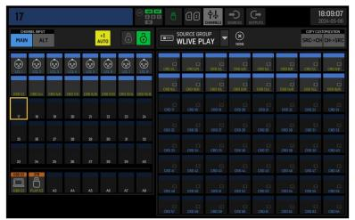
As a result from the operations above, Channel Strips 9 to 16 can now be used to mix the audio data issued from the first 16 tracks of SD card 1. Channel Strip 1 to 8 can still be used to mix the audio data coming from local inputs 1 to 8 at the back of the console, and Aux strips 1 and 2 can still be used to mix the audio signals from USB 1 & 2 and the 2 tracks from the USB stick player.
