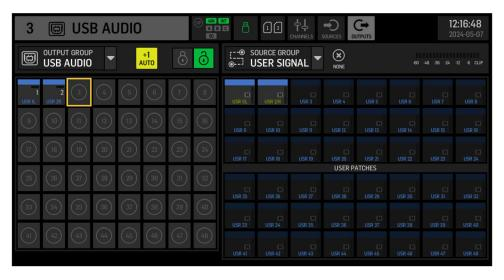
We can then hit play on WLIVE sessions on both SD card 1 and 2, and will get our signals available as a single stereo pair for recording a 2-track session over USB cable to a connected PC.
