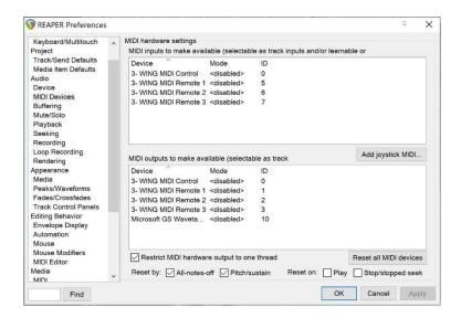
In the case of DAW control use, all WING MIDI devices above must remain <disabled> in the REAPER MIDI Devices panel to be used as a control surface communication MIDI device; REAPER will report errors otherwise.
