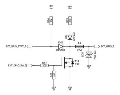
From the schematic above, we can see a 470 Ohm resistor in series with a diode and a 500mA poly-fuse going to the GPIO port. A max current of approx. 100mA is therefore available for connecting a small relay or an LED. TVS diode D70 protects against electrostatic discharge (ESD).
