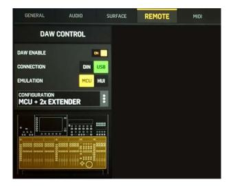
Transport controls proposed here include REW, Fast Forward, Stop/Play/Pause, Scrub, Jog Wheel and more, directly from the lower section of the WING controls. A simple/classic example of implementation is shown below and the setup of these functions is performed after pressing the WING controls' View button and assigning keys one by one using the WING main LCD screen.
