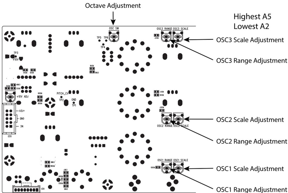
The diagram below shows the keyboard notes that are used in the calibrations. Only A2 and A5 are used in the Oscillator calibration, and C6 is used in the Octave calibration.
