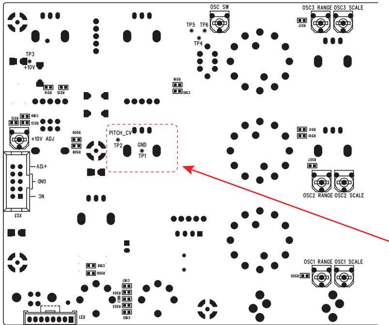
The diagram below shows the adjustment trimpots that are used in the Oscillator and Octave range calibration procedures. Take a look at your PCB and locate these various trimpots. (The later version of the PCB uses different multi-turn trimpots.)
