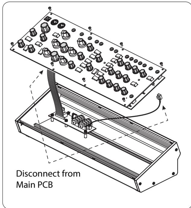
3. Disconnect the two cables from the lower side of the main PCB of the MODEL D, and remove the assembly from the chassis.
