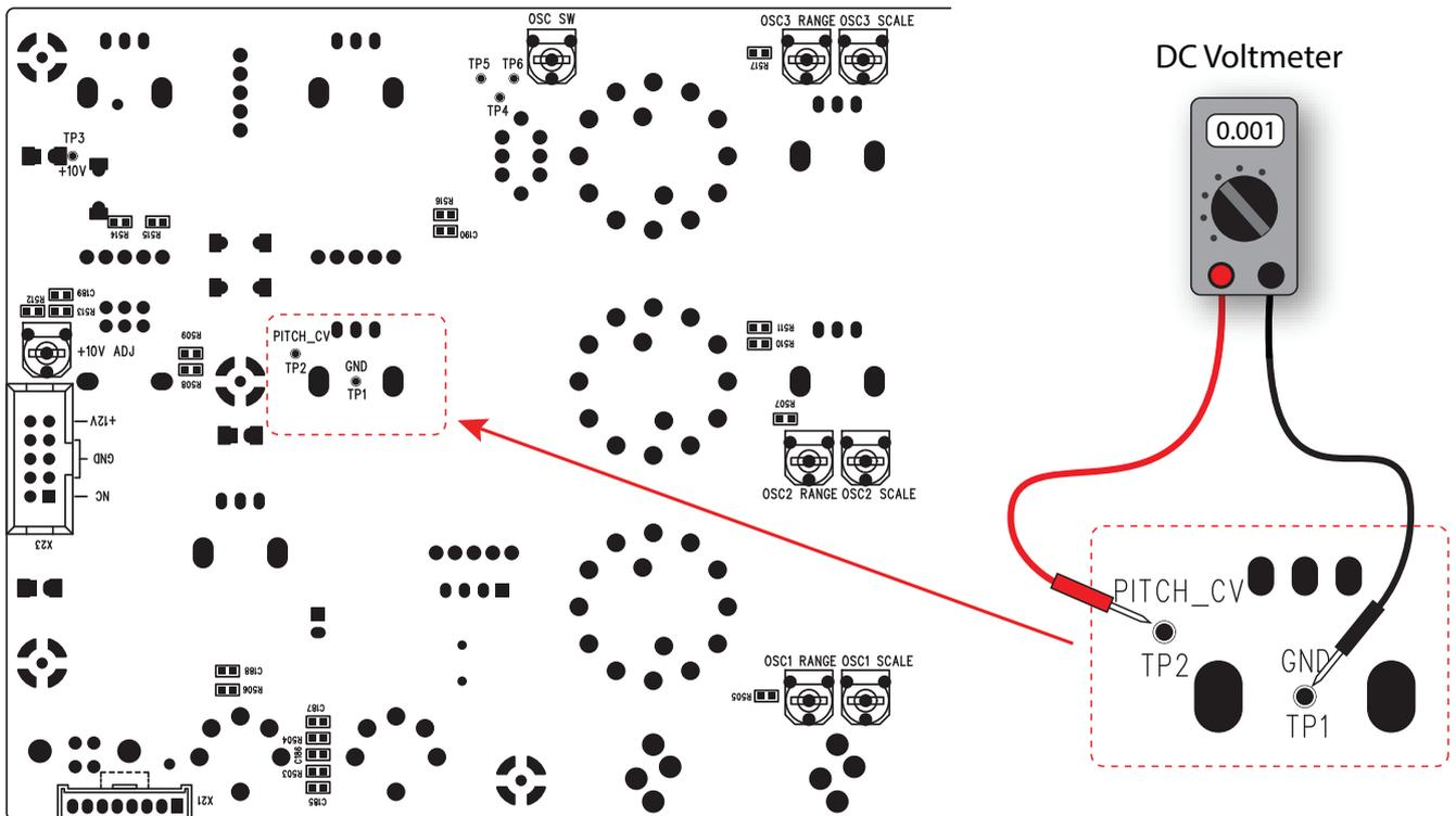
7. The keyboard diagram on the next page shows the keys used during the PITCH CV calibration procedure. The calibration requires setting three values: Low, Zero, and High. Various keys on the external keyboard are used to select and trigger these three different calibrations, to adjust the voltage readings, and to **Save** and **Exit** the procedure..
