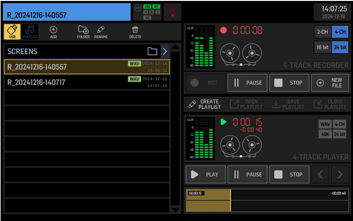
Figure 78: USB Recorder screen
