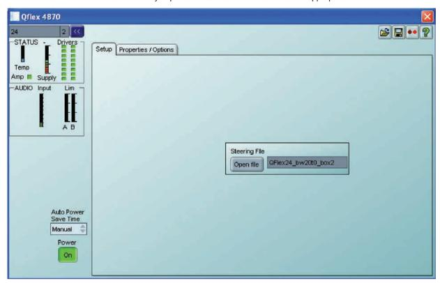
Note that when steering data is loaded into a loudspeaker, the data has to be stored internally, which takes a finite time. To avoid loss of steering data, do not remove the power from a loudspeaker for at least ten seconds after loading steering data. The same applies if you are loading a .dse Settings file which has steering data embedded into it.
