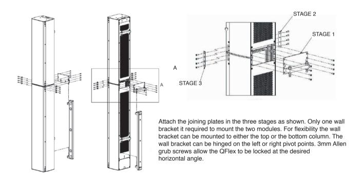
Having the hinge points on either side of the QFlex column allow the loudspeaker to be rotated at 90 degrees to the mounting structure allowing easy access to the input connector panel.
