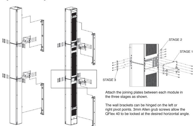
Having the hinge points on either side of the QFlex column allow the loudspeaker to be rotated at 90 degrees to the mounting structure allowing easy access to the input connector panel.
