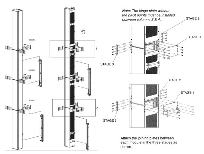
The wall brackets can be hinged on the left or right pivot points. 3mm Allen grub screws allow the QFlex 40 to be locked at the desired horizontal angle. The installer must ensure that the mounting surface is capable of safely and securely supporting the loudspeaker. Seek help from architects, structural engineers or other specialists if in any doubt.
