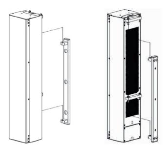
Having the hinge points on either side of the QFlex column allow the loudspeaker to be rotated at 90 degrees to the mounting structure allowing easy access to the input connector panel.
