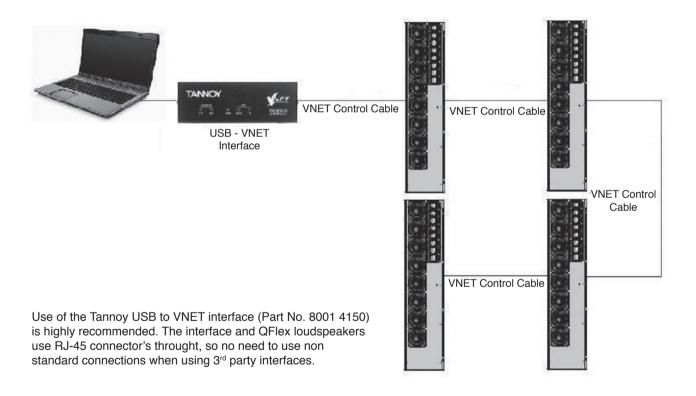
The VNET network uses the RS-485 protocol for sending serial data. It uses a pair of wires to send a differential signal over distances up to 4000 feet (1200m) without a repeater. The differential signal makes it very robust, RS-485 is one of the most popular communications methods used in industrial applications where its noise immunity and long-distance capability are a perfect fit.
