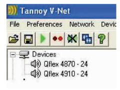
If PodWare becomes unable to communicate with a device for some reason whilst on-line (such as a break in the network cable), the corresponding icon for it in the Devices node of the Tree will appear in red, indicating that control and monitoring on that device is invalid. Most devices will allow themselves to be 'rediscovered' automatically if such a cable break is repaired.
