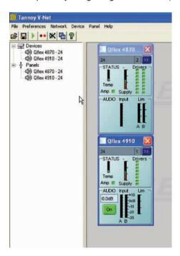
Several control panels may be launched onto the Layout, so that the user can monitor the operation of several devices simultaneously. As each panel is added, another icon is added to the Layout node of the Tree, indicating the presence of another panel in the Layout.
