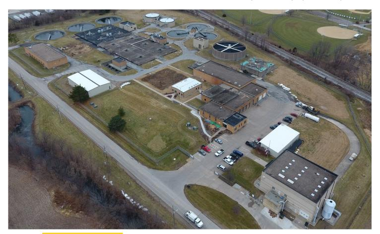
Population ~24,000 5.5 MGD average daily flow Trickling filter and activated sludge Two anaerobic digesters ~1M gallons
