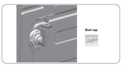
Step 1) Remove the dust cap.
