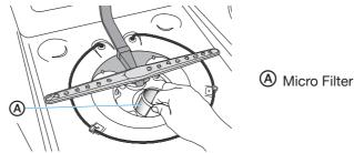
**6.** Inspect both the Fine fil er and the Micro fil er for debris, and then clean them by holding the fil ers under slow running water.
