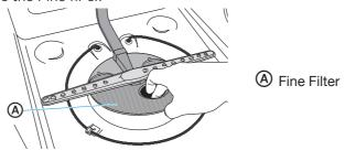
5. Remove the Micro fil er from the bottom of the tub.
