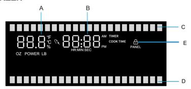
A: Microwave cavity display B: Time of cooking / timer / clock display C: Function prompt area
