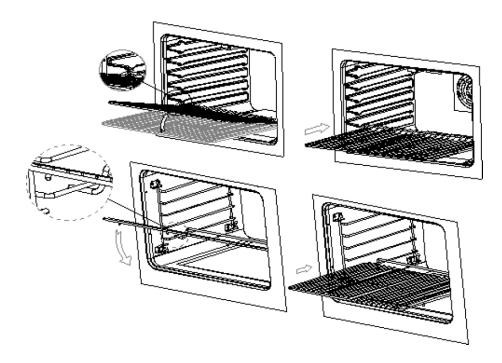
5. Lift the front about  $15^{\circ}$  upward till the tag of the shelf clears the safety stop of the side rack. Then lower the shelf horizontally and slide all the way into the oven. Other shelves can be installed this way.
