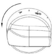
• To light the oven burner, push and turn the appropriate control knob counter clockwise to the (150 F~500 F) position. You will hear a clicking noise – the sound of the electric spark igniting the burner. Once burner ignition has been achieved, then turn the burner control knob to adjust the desired heat setting.
