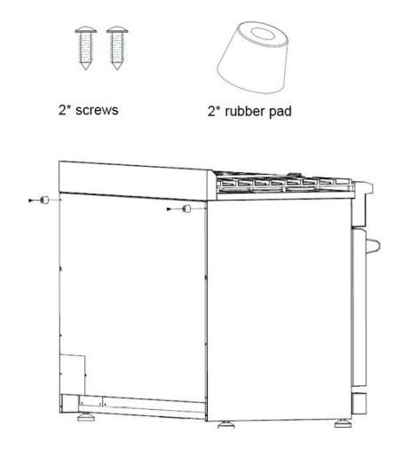
2. Install the 2 rubber pads as shown above.
