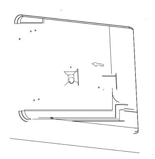
When replacing bulbs, release the glass cover on the lamp holder first, and then remove the bulb to replace with a new light bulb.
