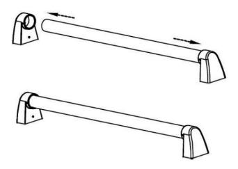
4.3 Lay the door handle against to the oven door and fit it on the connection part, and use the wrench to get the door handle holder tight;
