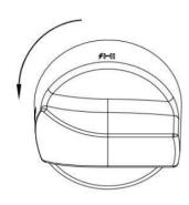
• To light the top burners, push and turn the appropriate control knob counterclockwise to the "HI" position. You will hear a clicking noise – the sound of the electric spark igniting the burner. Once burner ignition has been achieved, then turn the burner control knob to adjust the desired heat setting.
