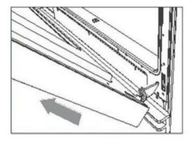
4. Disengage the hinges and remove the door, gently closing it about halfway. Place door on a protected surface.
