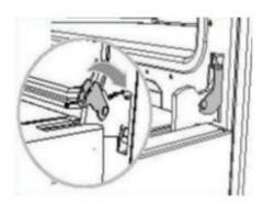
Fully close the levers on the left and right hinges, as shown, then close the door.
