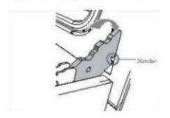
Insert the hinge tongues into the slots making sure that notches on both sides drop into place as shown.
