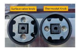
(Incorrect knob caused broken thermostat shaft)
