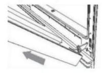
4.Take apart and remove the hinge, close it gently about half way through the door, and place it on the protective surface.
