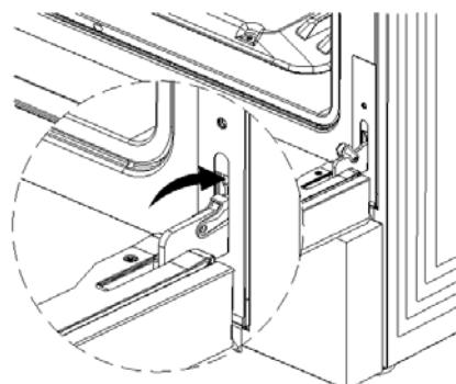
4. Fully close the levers on the left and right hinges, then close the door.
