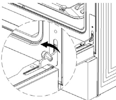
4. Disengage the hinges and remove the door; gently close it about halfway; place the door on a protected surface.
