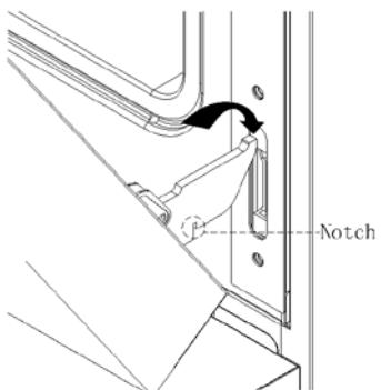
2. Insert the hinge tongues into the slots making sure that the notches on bothsides drop into place as shown.
