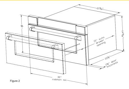
Figures 1 and 2 contain many Microwave Drawer measurements for reference when planning the drawer's location .This Microwave Drawer can be installed below
