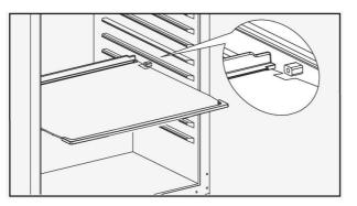
For easy access to the storage content, you must pull the shelves approximately 1/3 out of the rail compartment.
