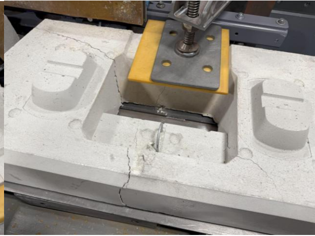
Figure 4 – Broken bottom block
