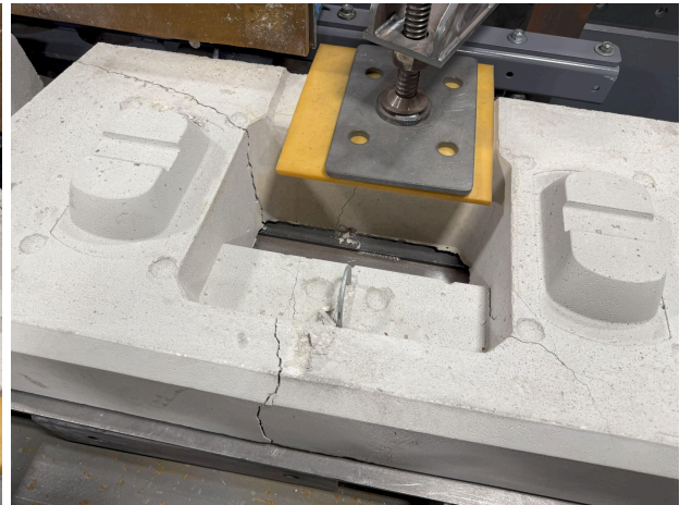
Figure 4 – Broken bottom block
