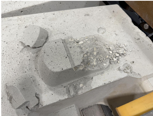
Figure 3 – Broken shear knob
