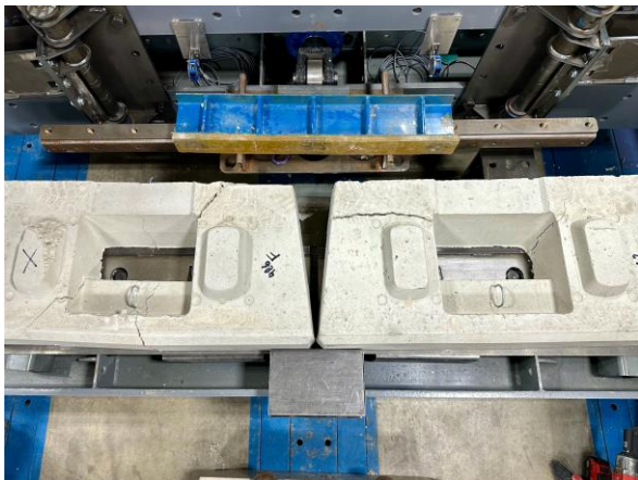
Figure 5 – Broken bottom blocks
