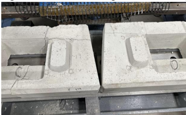
Figure 6 – Broken bottom blocks
