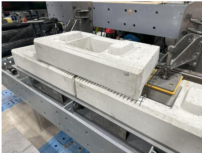
Figure 3 – Interface shear with geogrid inclusion test setup
