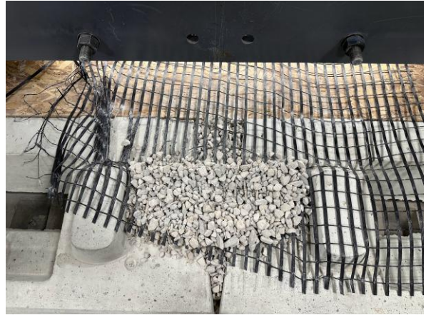
Figure 4 – Geogrid elongation and rupture
