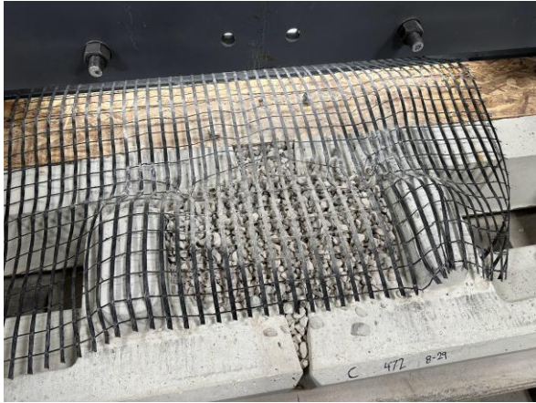
Figure 3 – Geogrid elongation and pullout
