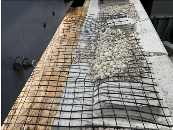
Figure 3 – Geogrid elongation and pullout
