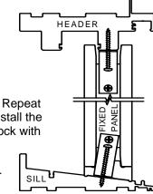
predrilled hole in the astragal bar, into the fixed panel, penetrating the aluminum reinforcement in the rail. Cover the hole with 3/8" hole plug.
