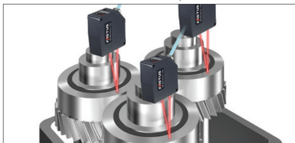
Flatness measurement of transmission parts
