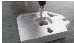
Needle contact-point mounting example
