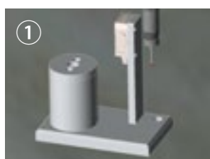
① The probe moves to the sensor of the stylus cleaner.
