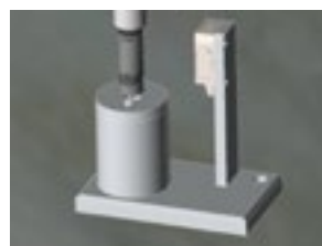
The probe moves the cleaning unit up and down several times to clean the stylus with cleaning fluid and compressed air.
