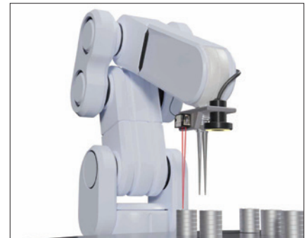
Stacked Bearing Height Measurement
