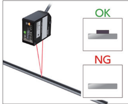
Detecting seal material on pressed products
