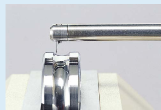
Inner/outer ring contour of a bearing
