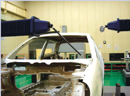
Measurement example for dual-arm type (Simultaneous use of touch-trigger probe and line laser probe)
