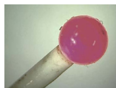
Contaminated stylus tip
