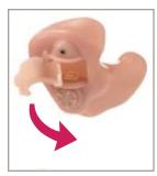
**NEVER FORCE THE DOOR SHUT.** This could result in serious damage. If the door will not close easily, check that the battery is placed properly in the compartment and is not upside down.
