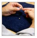
Use the cleaning brush/ waxloop and/or a soft, dry cloth to remove earwax or other particles that may accumulate around the canal, volume control, and battery compartment; never use water, solvents,
