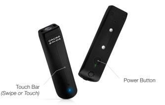
OrCam<sup>®</sup> MyEye is a device that is used by visually-impaired persons to help them interact more effectively with the world. OrCam can recognize and read text, identify currency, learn and recognize faces, identify products and more. When paired to a compatible hearing aid, the audio from the OrCam MyEye is streamed wirelessly to the hearing aid.
