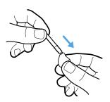
Pull the application stick straight out to remove the used wax guard. Do not twist.
