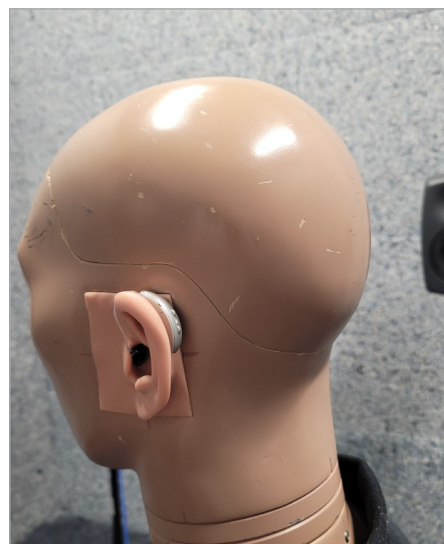
Figure 3: GRAS KEMAR wearing an Aris AI RIC hearing aid used in this study.
