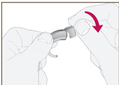
To access, remove the battery with the DAI shoe attached:
