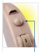
BTE's with a telecoil feature enable you to comfortably use the telephone without removing your instrument or earmold. The induction coil amplifies the signal emitted naturally from the telephone receiver.
