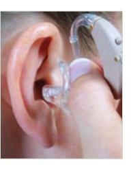
To insert, hold the earmold with your thumb and forefinger on the outer side near the tubing. Gently insert the canal tip of the earmold into your ear canal. Then softly press the earmold into place with your fingertip.
