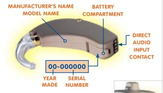
Your BTE has a tamper resistant locking battery compartment. The lock switch is located on the bottom of the battery door.
