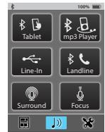
(2) Audio sources, available for selection, are displayed. To turn on audio streaming, select an audio source button, which then becomes highlighted. To turn off audio streaming, select the highlighted audio source button.
