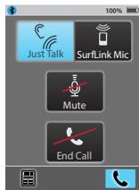
(3a) Either **JustTalk** (uses the hearing aid microphone) or **SurfLink Mic** (uses the built-in SurfLink Mobile 2 microphone) can be used to pick up your voice during a phone call. Select desired voice input option by toggling between JustTalk and SurfLink Mic.
