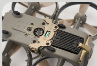
Loki MkII sUAV Payload Connection Bracket
