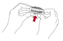
4 Keeping your hand away from the blast doors, place the cartridge into the front of the energy weapon until it is approximately 90 percent inserted.
