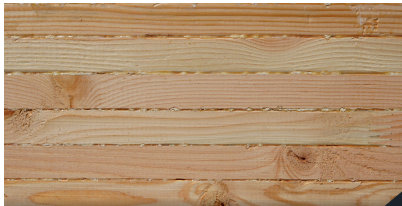
Framing Appearance Beam
