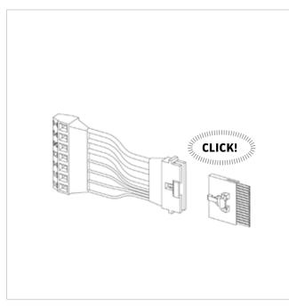
Plug connections must always click into place. Press the latch to unlock.
