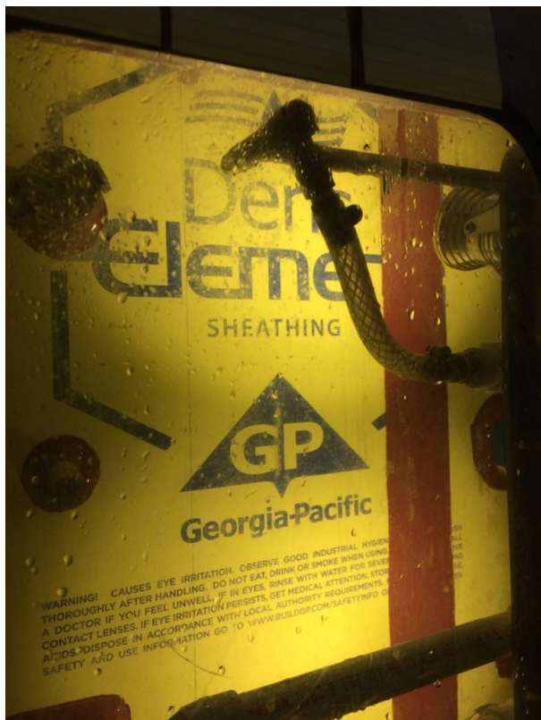
Picture: The DensElement ® Barrier System tested per ASTM E331.
