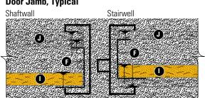
**Door Jamb, Typical with Jamb Anchor Clips**
