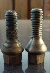
The HYTORC Gall-Free Nut coated thread design eliminates the microscopic material corrosion that occurs when fasteners are subjected to high temperatures and increased friction over extended time periods. This technology counters the galling effect of plastic deformation and micro-scale material transfer of thread surfaces.
