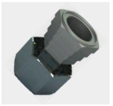
The two-part design consists of interlocking inner and outer sleeves with tapered threads that integrate advanced anti-galling properties. Compatible with standard bolt threads, the HYTORC Gall-Free Nut can be finished in a variety of coatings and materials to suit your specific applications.
