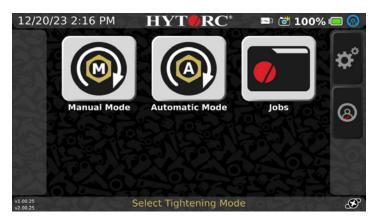
The start screen appears after switching on the pump.
