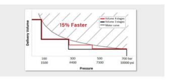
By adding a 4th pressure stage in the 4,000 to 7,000 psi range the HY-115/230 Pump increases the flow of oil to the tool. Allowing the tool to cycle faster and resulting in a 15% time savings over old 3-stage pumps.
