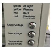
The HY-115 Pump is equipped with three-colored (3) LED lights integrated into the electric control box for system monitoring. The LED lights let you know that you are operating within voltage and temperature limits.
