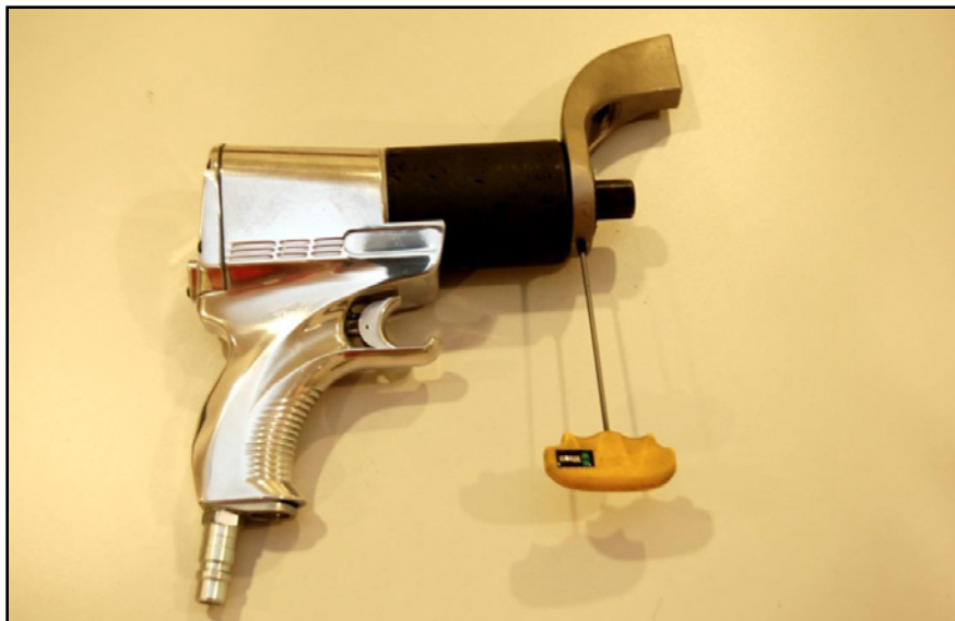
Figure 5. Tightening Reaction Arm Set Screw
