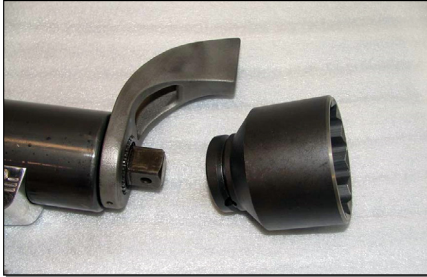
Figure 6. Installing jGun Socket
