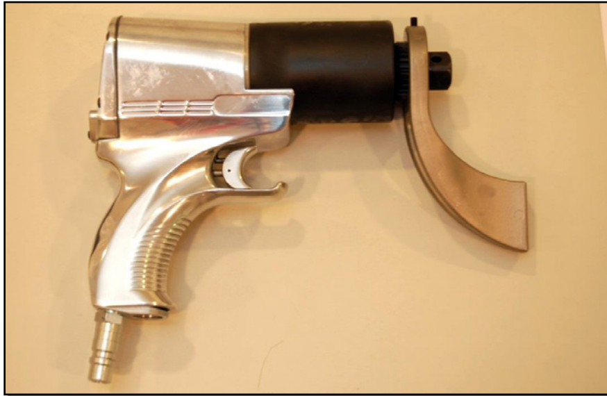
Figure 4. Reaction Arm installed
