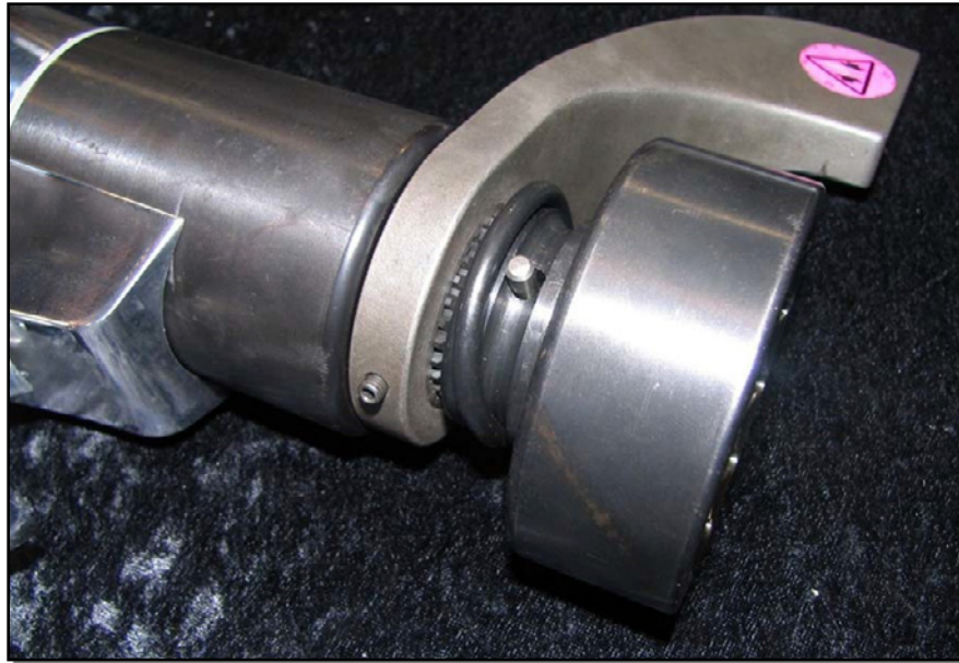
Figure 7. Installing Socket Locking Pin and Retaining Ring
