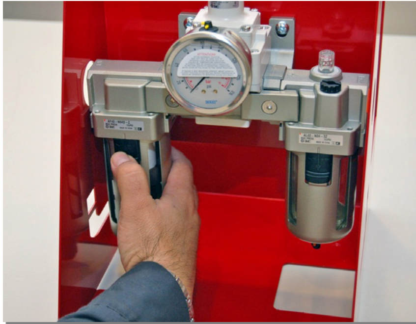
Figure 15. Emptying the FRL Filter Reservoir
