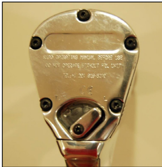
Figure 9. jGun Drive Direction Lever
