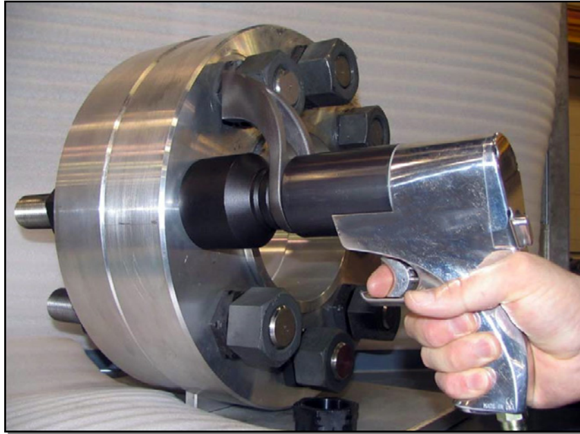
Figure 11. Using the jGun with a HYTORC Washer
