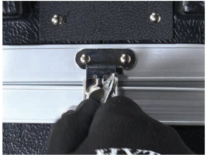
Close case: Close covers until properly aligned (studded plates must match up), then turn butterfly keys until case is flush and keys no longer rotate.
